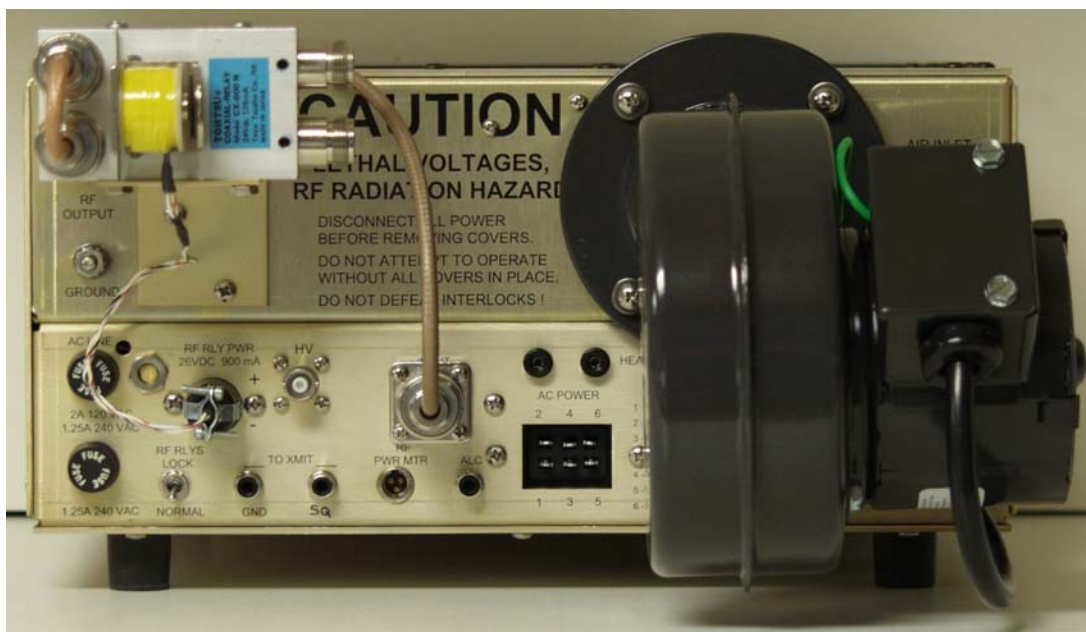
Rear View of a LA-x2A RF deck with blower and relay package installed.
